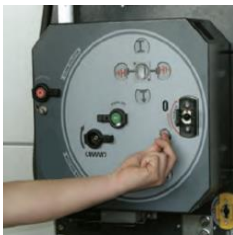
7- Lock the air rotary isolator by the key (if available)
