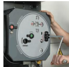
6- Lock the air rotary isolator in “open” position
