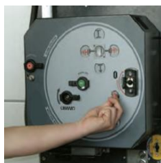
5- Unlock the air rotary isolator by the key (if available)
