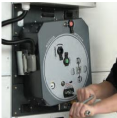
4- Unlock the air rotary isolator
