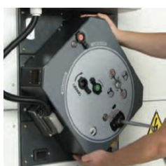
7- Close the air rotary isolator by the rotation
