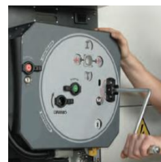
6- Unlock the air rotary isolator
